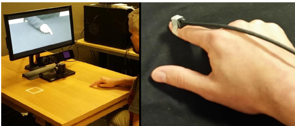
Figure 2: The experimental set up. The computer displaying the videos with the eye tracker in front (left image) and motion sensor (right image).
